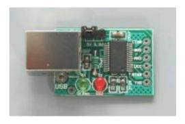
This converter provides two way serial communications signal conversion between the TTL (Transistor Transistor Logic) output to and from a personal computer USB port using virtual serial COM port.
