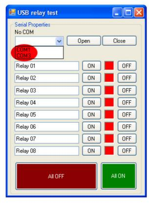
4. Choose COM port. Click on "OPEN" button and using "ON" and "OFF" buttons you can test relays.
