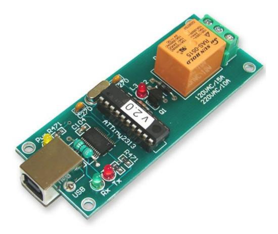
A general purpose USB Relay board (controller) for connection to a PC's USB port using VCP (Virtual COM port). Control devices using your PC.
