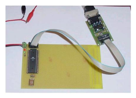
In order to use an ISP programmer, the target device must be powered and have a oscillator, as the programmer has to communicate with the target device under standard operating conditions rather than a specific programming mode.
