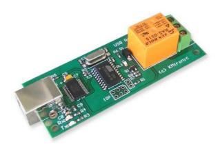
A general purpose Relay board for connection to a PC's USB port using VCP (Virtual COM port). Control devices using your PC. USB Relay controller allows a PC to control external devices using simple RS232 commands. Relay is fully powered from the USB bus.
